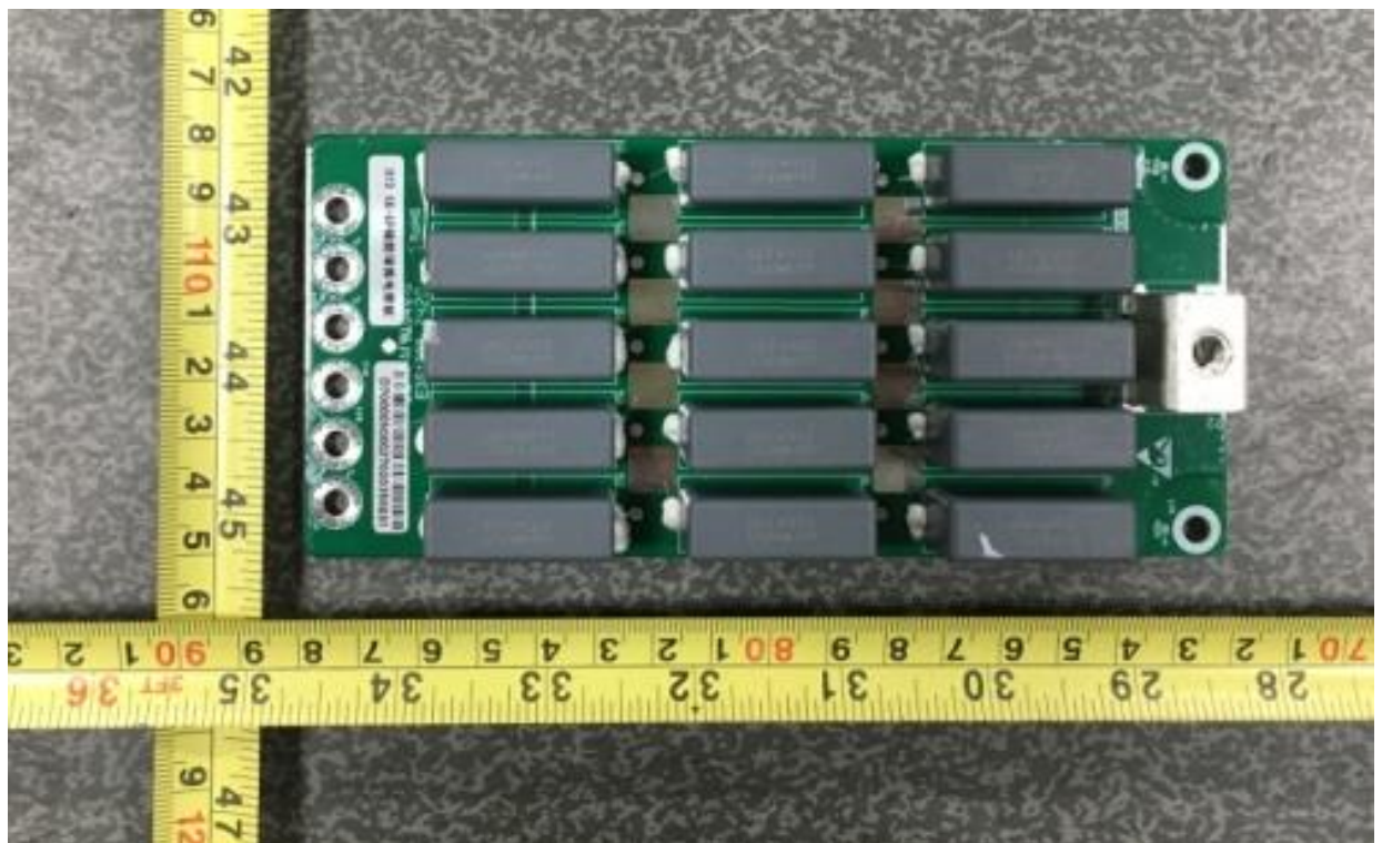
Filter board view (Components side)
